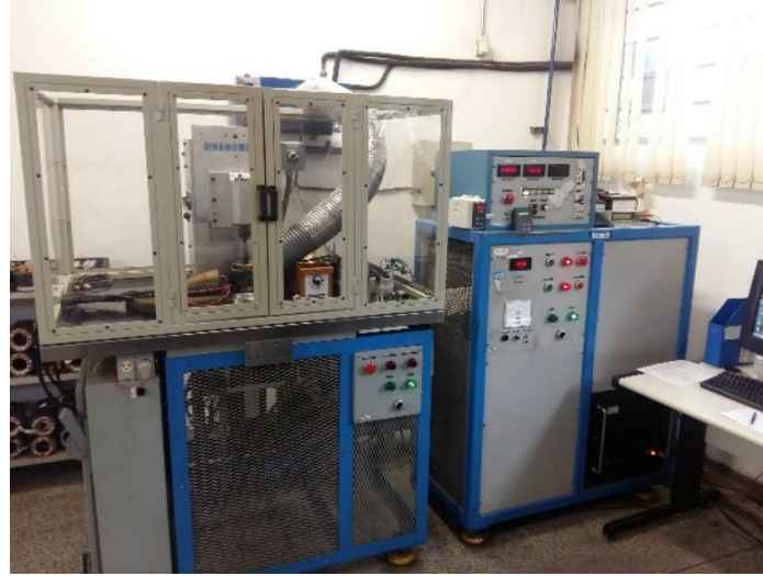
Figure 3: Servo motor dynamometer for motor characterization.
